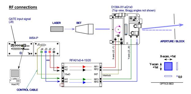
\*\* Note the specific connection order between the four iMS4 outputs to the RFA01x0-4 amplifier inputs.
