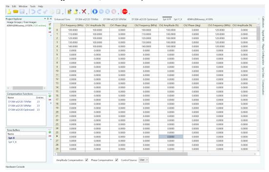
This table comprises 5 frequency points equally spaced across the maximum diffraction bandwith of the AOD.
