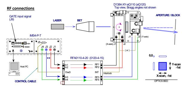
\*\* Note the specific connection order between the four iMS4 outputs to the RFA01x0-4 amplifier inputs.
